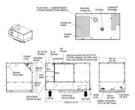
Note: This outline drawing is provided for general reference only and is not intended for design or installation. For more information see Operation and Installation manuals or obtain drawing 500-4040 and wiring diagram from your distributor/dealer.
